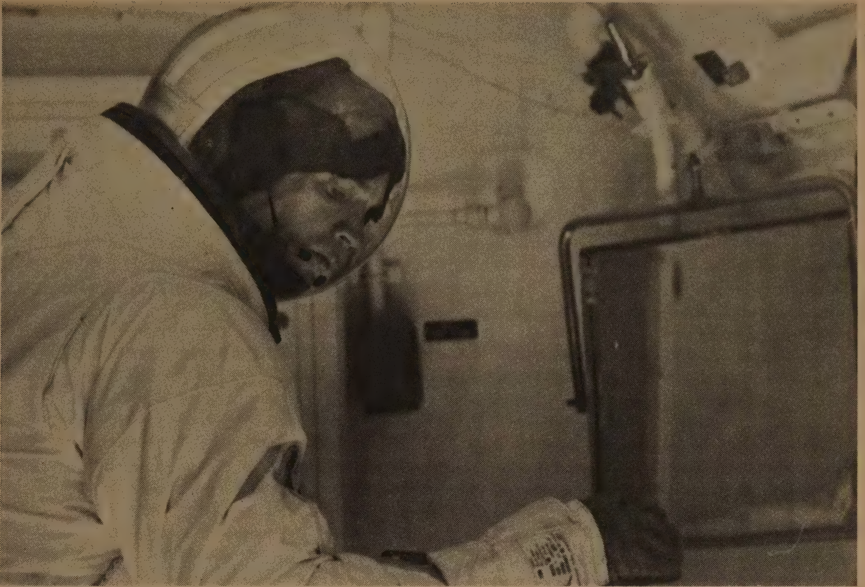
June 1968, Houston. Schweickart at a simulated altitude of 200,000 feet testing the Portable Life Support System which makes his suit an independent space vehicle. With it he made the first spacewalk without an umbilical.
